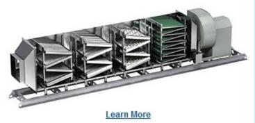
The Grease Trapper uses a three-stage mechanical filter arrangement to remove grease and smoke particles from the exhaust air of a restaurant at an economical first cost. Activated carbon panels remove odor molecules prior to discharging the air, reducing the impact of kitchen exhaust to the surrounding areas.
